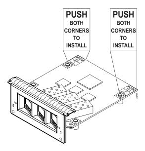
Step 4 Press gently on the white labels in middle of the outer edge of the EPA as shown in Figure 13 to ensure that the connector is fully seated.
